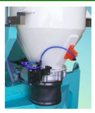
As we said, the next step is to weigh the materials and then be able can mix them. For this purpose we are going to use a programmable weighing machine. According to the type of concrete, we will weigh the exact quantity of material that we need. The PLC will receive an analogic input and when it reaches the necessary value, the system will not dump more material.
