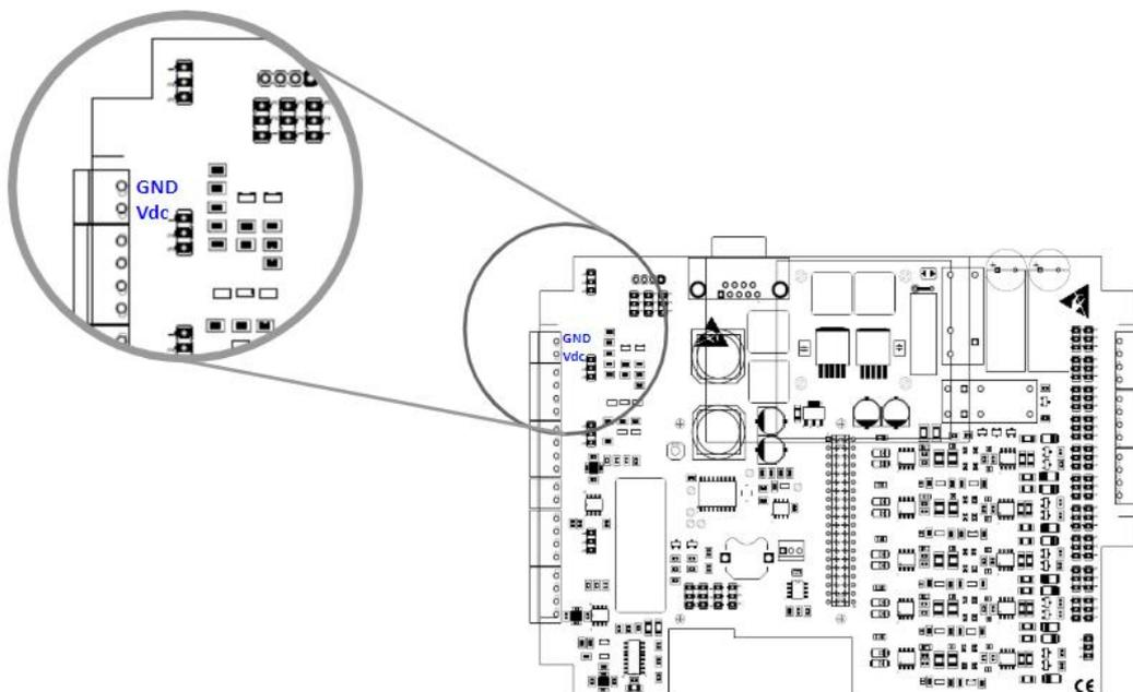
Find attached a picture regarding the position of the external power inputs:
