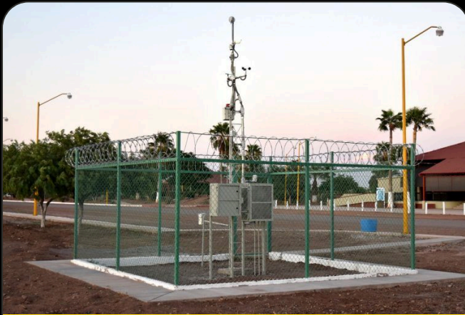
The weather station in the Yaqui Valley, Mexico: sensor mast and field cabinet.
