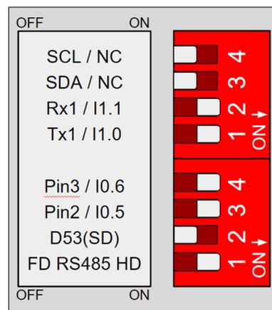
**4. SCL/I2.1: ALWAYS AT OFF POSITION.** On the MDUINO PLC ARDUINO ETHERNET 38AR I/Os ANALOG/DIGITAL PLUS Controller this switch is **not connected**.
