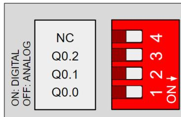
For the Relay Shield if a switch is set to ON, it can only act as Digital Output. If it is set to OFF it can only act as an Analog Output.
